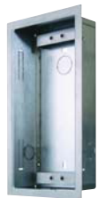
9135351E Flush fixed box for 1 module 125 x 235 x 46 mm Hole: 110 x 220 x 50 mm
